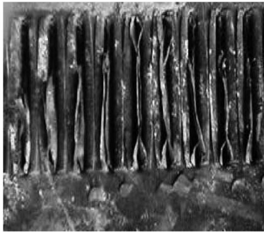
Example 2: PPL separated from base metal due to sulphuric acid attack
